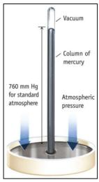
We measure atmospheric pressure with a **Barometer**:
